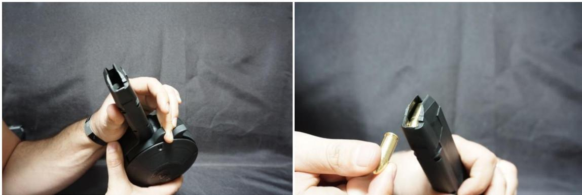
*While keeping the spring compressed, slide a cartridge primer, end first into the gap created.*
