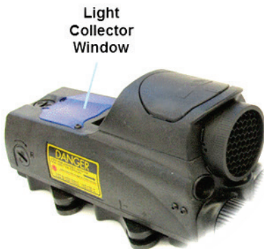
Figure 2: Light Collector Window (Cover)
